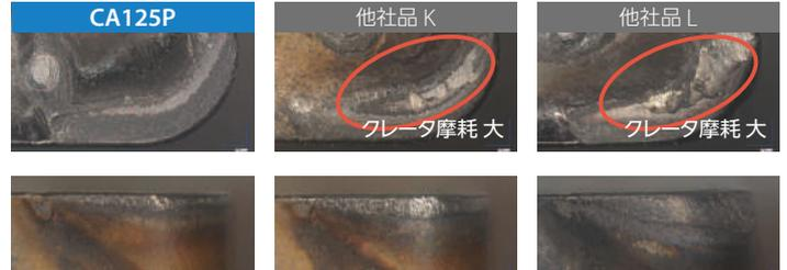
切削条件: Vc = 300 m/min, ap = 1.5 mm, f = 0.3 mm/rev, Wet 被削材: SCM435
